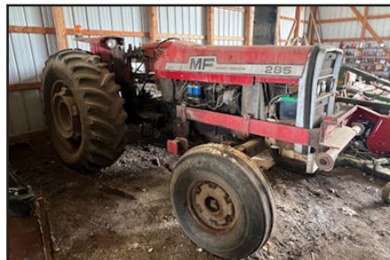
Massey Ferguson 285 Diesel Tractor, 18.4-34 Rear Tires, 3 pt. PTO 540, 1619 Hrs.
