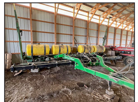
JD 70000 Planter, 8 Row 30", Liquid Zone Tiller Fertilizer, Herbicide / Insecticide, Box Extensions, Dickey John Monitor
