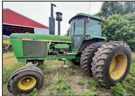
JD 4840 Tractor, 3430 Hrs, Powershift, 20.8 R 38 w/ Hub Duals, Triple Hyd., 1000 PTO S/N: 004347R
