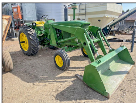
JD 4020 Diesel Tractor, 8400 hrs, 3pt, Dual Hyd, 540/1000 PTO, Syncro Range, 16.9/14-34, JD L148 Loader
