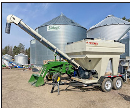
Friesen 240 Tandem Axle Seed Tender, Honda 5.5 hp Engine
