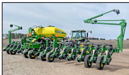
JD 1770 NT 16 Row 30" Vacuum Planter, CC5 Seed Delivery, Pneumatic Row Unit Air Bags SN:TCM750121
