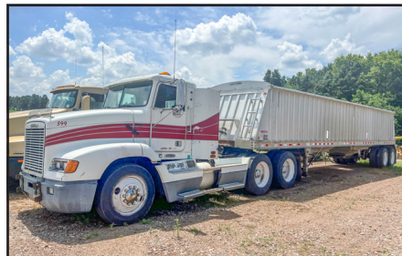
1999 Freightliner Semi Tractor, Eaton Transmission 10sp, C10 CAT 285/75R 24.5 Tires Dakota 38' Semi Trailer, Roll Tarp, Aluminum Frame, Ag Hoppers, 285/75R24.5 Tires
