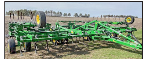
JD Model 2230LL 43" Field Cultivator, 4 Bar Harrow, Knock on Sweeps, Heavy Shanks
